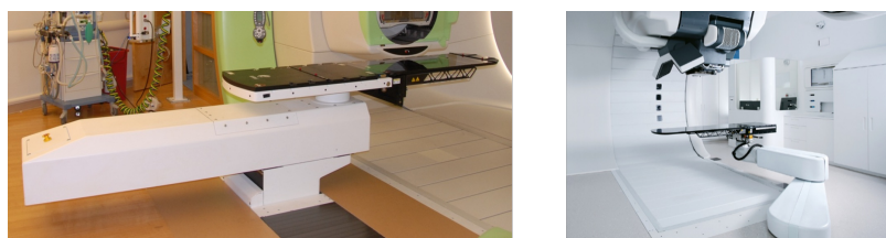
Figure 16. Two typical proton therapy treatment couches. The couch on the right is a robotic version.
